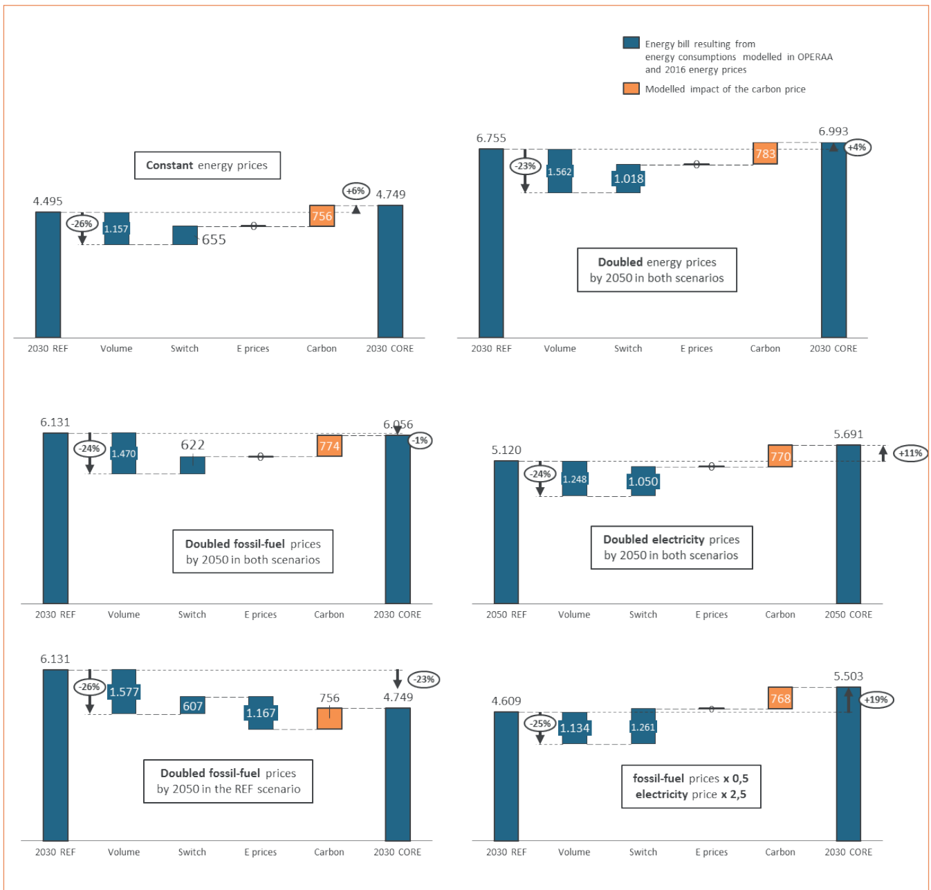
A.3.17: Annual energy bill for heating non-residential buildings by 2030 in the BaU and the low-carbon scenario with different assumptions on the evolution of energy prices [€/household/year]
